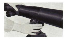
Focusing can be done by turning the knob at the bottom of the lens as shown in the photo A.
